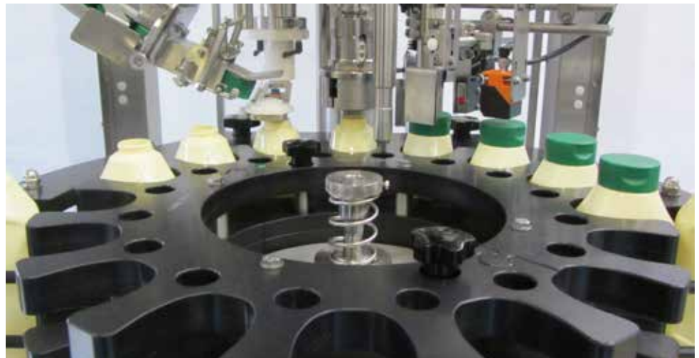
SCREW-CAPPER FOR PLASTIC CAPS ONTO PET BOTTLES FOR KETCHUP
