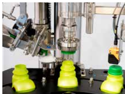
Single capping head for: screw-capping (with jaws or chucks) or sealing, or push-down capping
