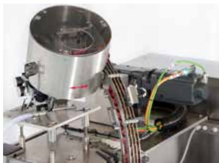
Universal cap sorter type D300 for caps 30mm in diameter. Stainless steel cap chute with cap dispenser and direct cap pick-off.
