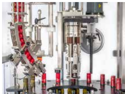
One sealing head in either bronze or stainless steel (upon request).
