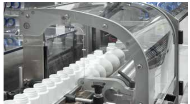
BOTTLES MOVING ON CONVEYOR TO CAPPING STATION
